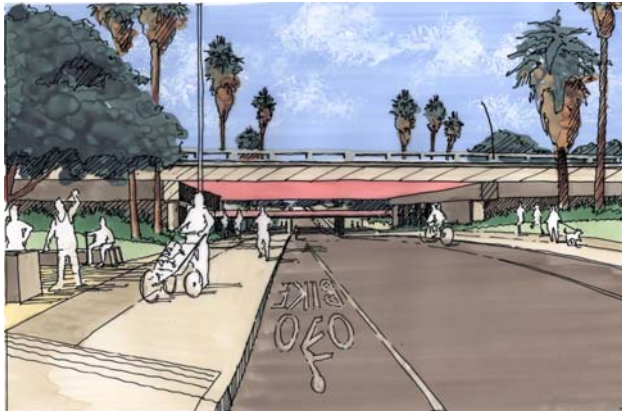
Under Interstate 610 the sidewalks are widened for pedestrians, bicyclists, joggers etc. Overgrown vegetation is removed for safety. Palm trees and lighting are added to mark the crossing of the park and the interstate.
