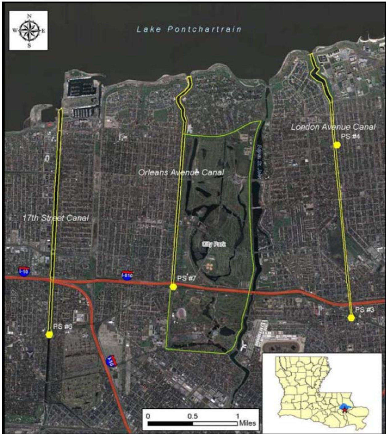
Figure 6 - Pump Station #7 and Drainage Outfall through Orleans Avenue Canal to Lake Pontchartrain (Yellow hexagons represent pump station locations)
